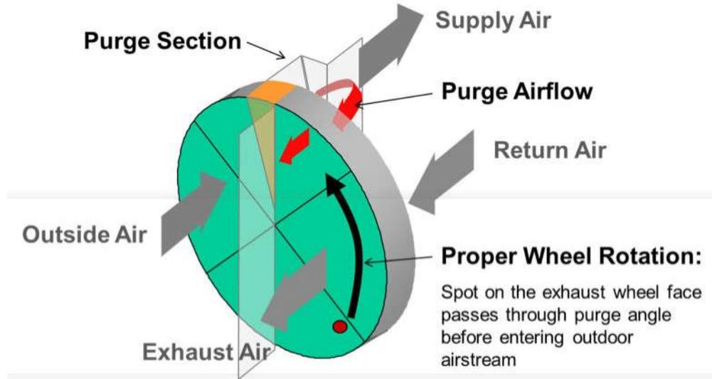
Figure 4 Illustration of the purge section and correct rotation direction for purge operation
