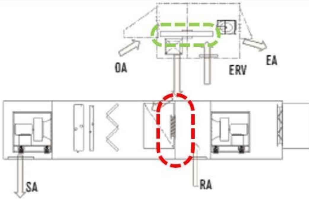
Figure 13 VAV AHU with Recirculation and separate ERV Unit
