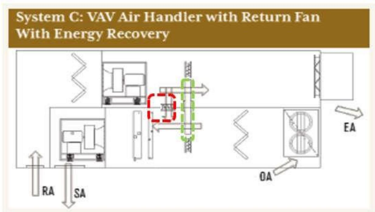
Figure 12 VAV AHU with Recirculation and ERV
