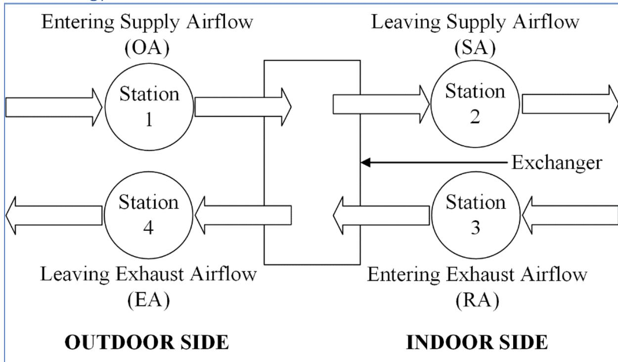
Figure 8 Standard Designation of Airflows at Exchanger
