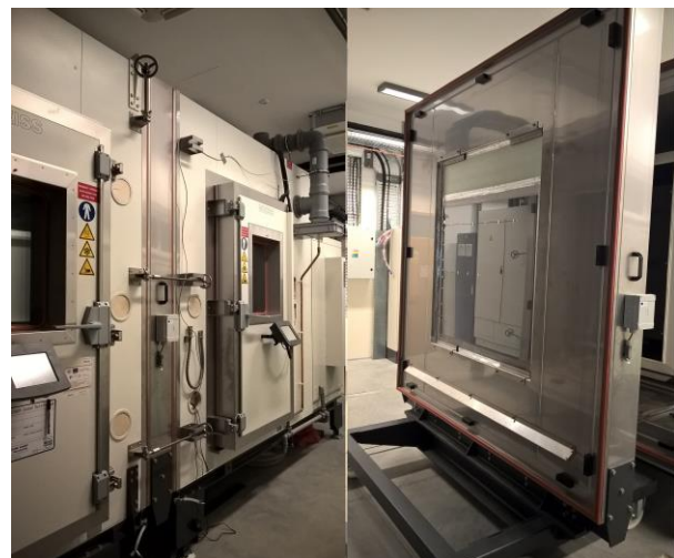
Figure 1 Climatic chamber used and integrated TIF prototype prepared for measurement
