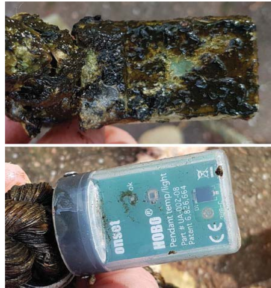
Figure 3: Example of organic aggregation on the loggers, as observed on the 22nd of September. The upper figure shows the upper sensor, the lower figure shows the second lowest one.
