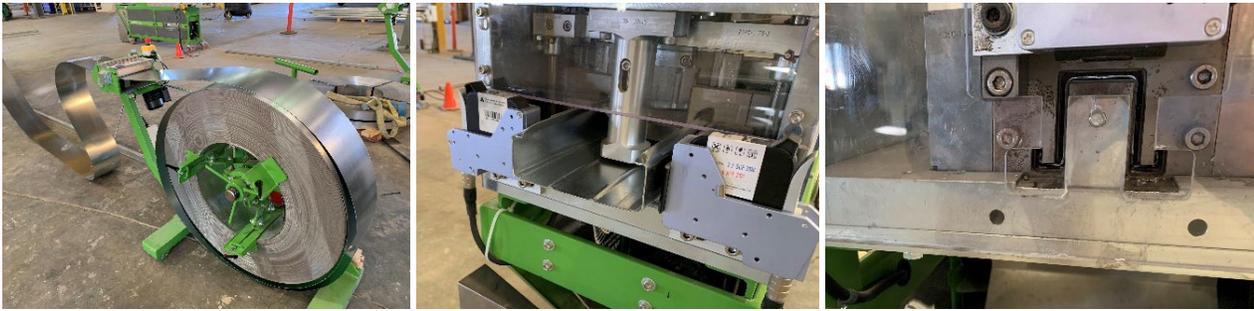
**FIGURE 5. TOP: LGS MACHINES TO PRODUCE WALL FRAMINGS, AND ROOF AND FLOOR TRUSS ASSEMBLIES. BOTTOM (LEFT TO RIGHT): LGS FEEDSTOCK AND LGS STRUCTURAL MEMBERS WITH DIFFERENT CROSS-SECTIONS RESULTS AND DISCUSSION**
