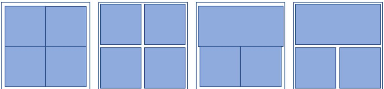
**Figure 1. VIP assemblies for evaluation of edge effects. The overall assemblies are 24" x 24" and the central measurement area is 10" x 10" (overlapping the VIP interfaces). Parameters for EnergyPlus models**
