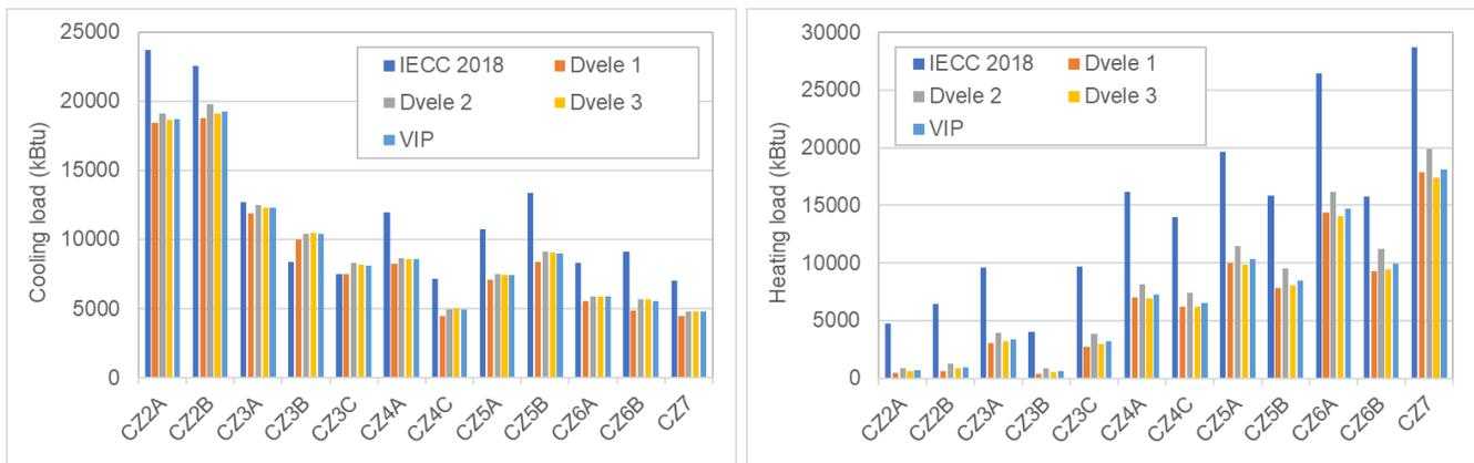
**Figure 8.** Calculated cooling and heating loads for the Roberts design with different envelope configurations across different climate zones.
