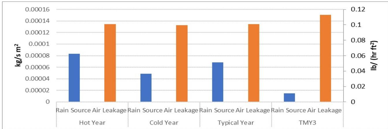
**Figure 3** Annual moisture deposition on the exterior sheathing for the typical residential wall in Arctic Alaska.
