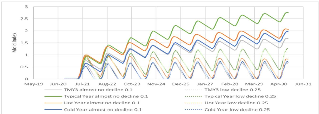
**Figure 4** Mold index (at the inner face of the exterior sheathing) for a wall representative of existing building stock across weather scenarios. The solid lines in Figure 4 show the data with almost no decline 0.1, which is the default for OSB in the mold model. The dotted lines are relative decline, 0.25.
