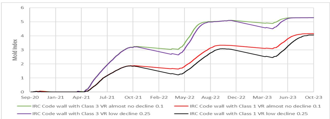
**Figure 5** Change in mold index over time for IRC-code-minimum retrofit scenarios. This data is for the interior layer of OSB that is directly beside the fiberglass.
