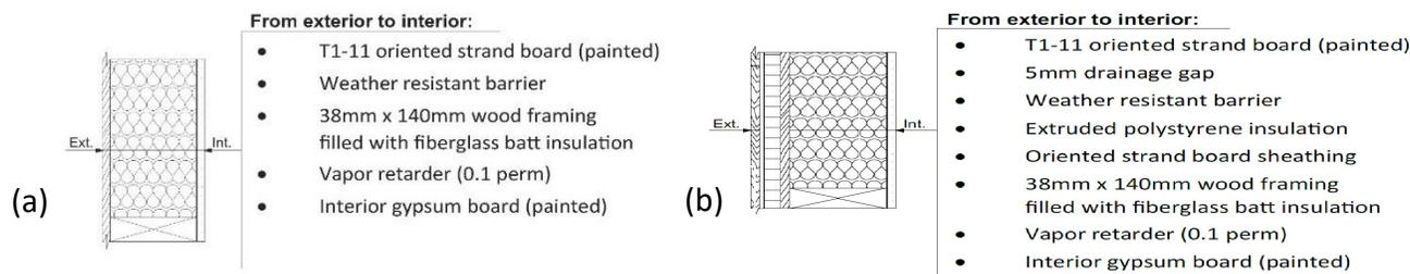
**Figure 2** Components of the evaluated wood-frame wall assemblies, (a) is typical to the North Slope Borough housing stock (nominal 2 in x 6 in frame cavity) and (b) is the IRC minimum retrofit wall (nominal 2 in x 6 in frame cavity).
