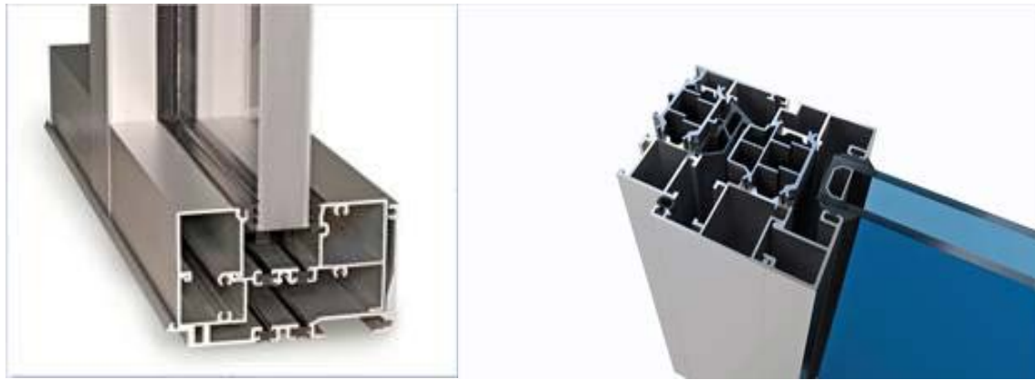
Figure 5-11 (EN18) Thermally Broken Aluminum Frames Double pour-and-debridge (left) and wide thermal struts (right) Photos courtesy of Azon (left) and Technoform (right)
