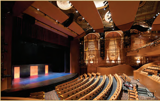
Figure 7 The Allen Theater at Playhouse Square. The original walls are covered by an acoustically and visually transparent material, allowing historical fabric to be augmented with modern lighting and technology systems. Source: DLR Group
