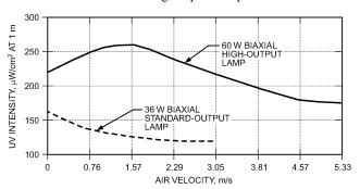
Fig. 5 Windchill Effect on Typical Low-Pressure UV-C Lamp Efficiency in Moving Airstream at 21°C
