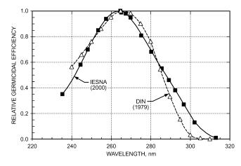
Fig. 1 Relative UV-C Germicidal Efficiency
