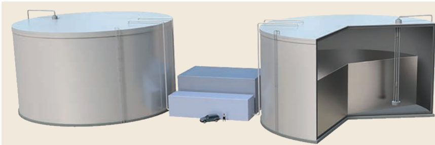
MIT researchers propose a concept for a renewable storage system, pictured here, that would store solar and wind energy in the form of white-hot liquid silicon in heavily insulated tanks.
