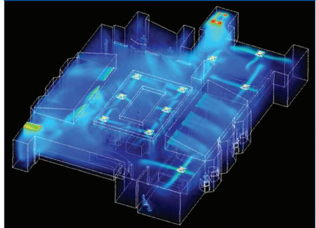
space volume and potential vertical air stratification, higher ceilings introduce larger volumes of air to condition and supply, and returns are further away from the occupant’s breathing zone. Filtration and purification provided by the central system will have to overcome these challenges.
