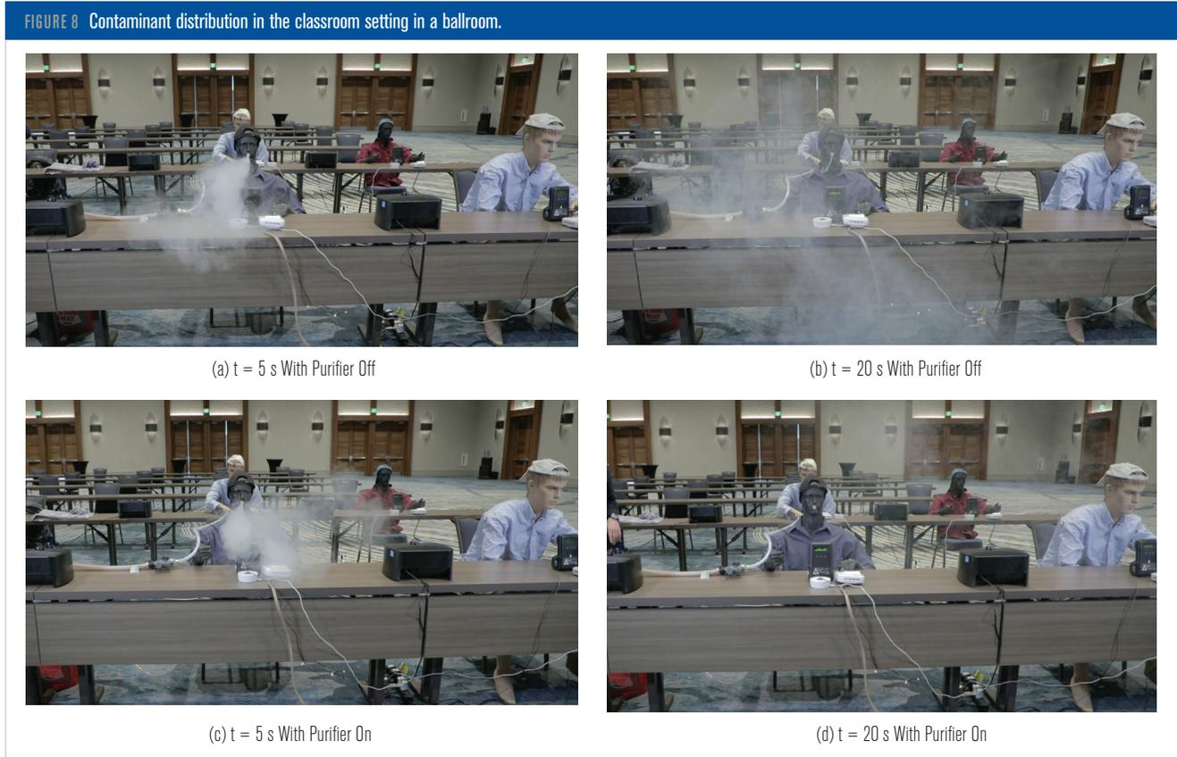
occupants, was able to contain the contaminant within the source premises and remove the contaminant in a timely manner. Similar dispersion patterns were observed for the banquet case. However, due to the size of the banquet table and occupant density in the banquet setting, air purifiers with proper inlet/outlet locations and flow rate need be further identified.
