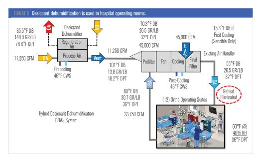
Of great significance in this example is that the need for costly "reheat" has been eliminated, which in conventional operating room design may range anywhere from  $15^{\circ}F$  to  $30^{\circ}F$  ( $-10^{\circ}C$  to  $4.0^{\circ}C$ ).
