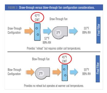
blow-through (cooling coil located after fan) configuration. This allows the residual motor heat from the draw-through fan to be used as a source to heat the airstream leaving the cooling coil, moving its final condition slightly off the saturation point (reducing relative humidity) usually enough to avoid any moisture condensation downstream. The problem with this design is that it may be less energy-efficient than an alternative design using a blow-through fan.
