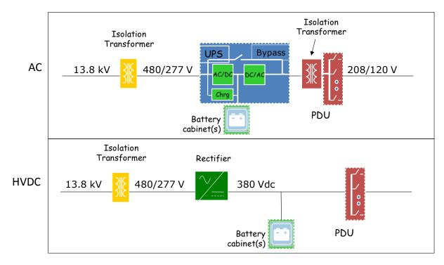
Figure 32 AC and HVDC Power Trains
