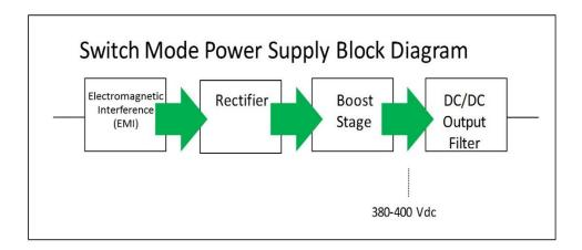
Figure 31 IT Equipment Power Supply Train
