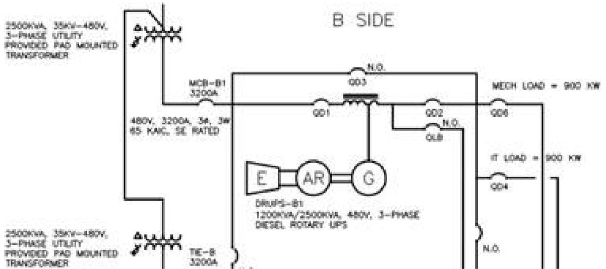
**Figure 2 – Typical Diesel Rotary Uninterruptible Power Supply (DRUPS) Topology – One-Line Diagram Depiction**
