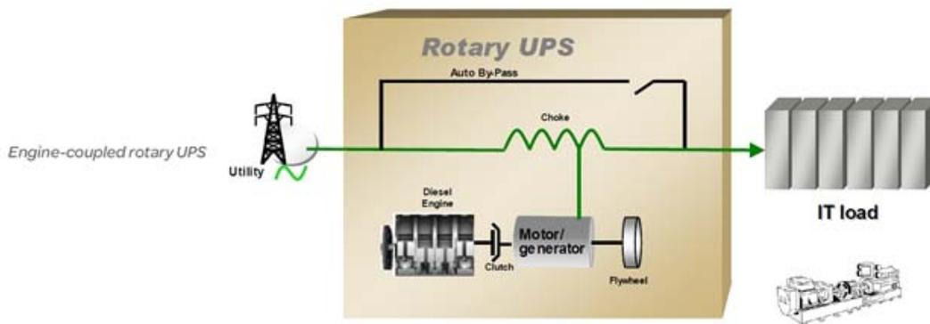
**Figure 1 – Typical Diesel Rotary Uninterruptible Power Supply (DRUPS) – Block Diagram**
