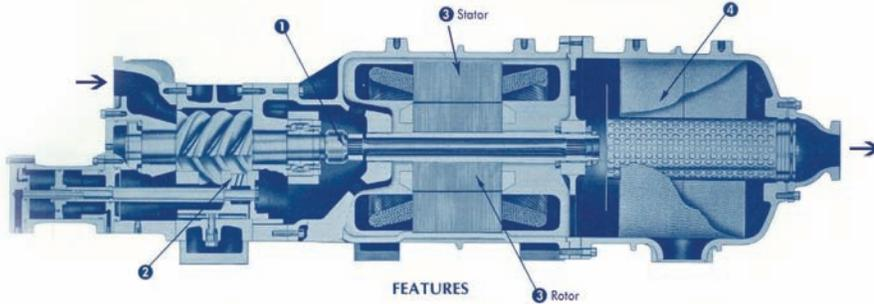
Figure 1: Design of first large hermetic screw compressors.
