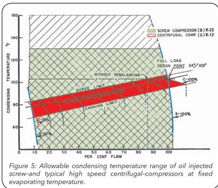
Figure 5: Allowable condensing temperature range of oil injected screw and typical high speed centrifugal compressors at fixed evaporating temperature.
