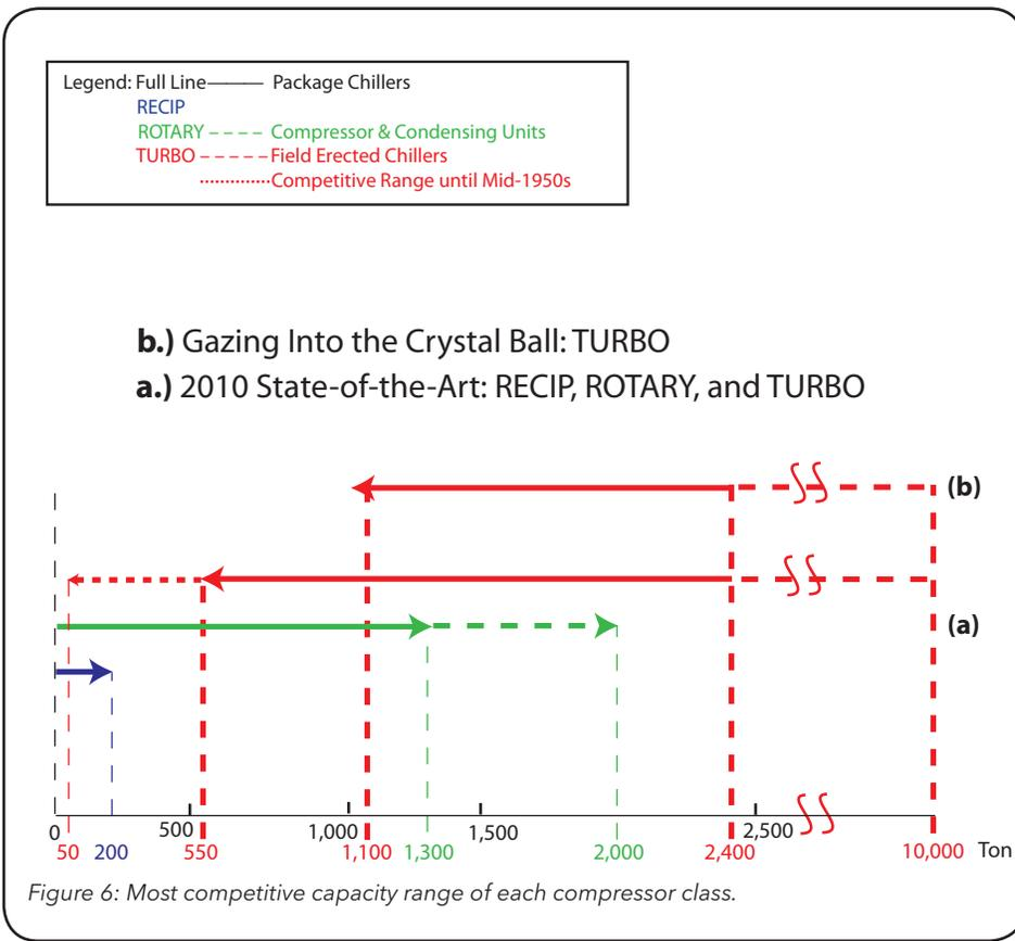
Figure 6: Most competitive capacity range of each compressor class.
