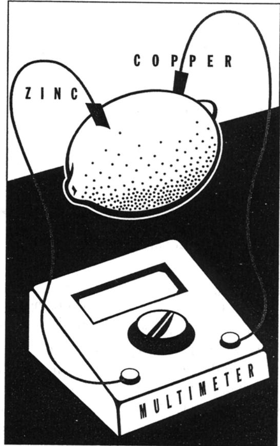
Chemical energy is the source of power in batteries. The simplest batteries consist of two different metals (electrodes) floating in a bath of acid. Atoms from one metal travel through the acid to the other metal releasing electrons. Eventually, when all the mobile atoms have been transferred, no additional electrons may be released, and the battery is dead
