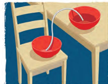
over the second container. Nothing will happen – there is no fluid in the tubing and nothing to make the fluid flow.
