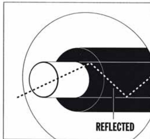
optical fiber, tie it in a knot, and light is still transmitted through it.
