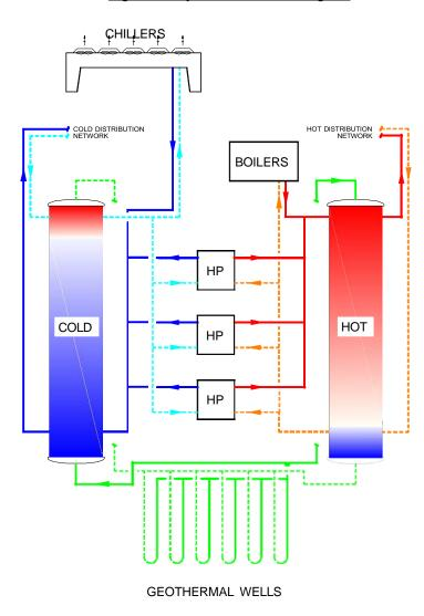
Figure 2 : Hydronic network Diagram
