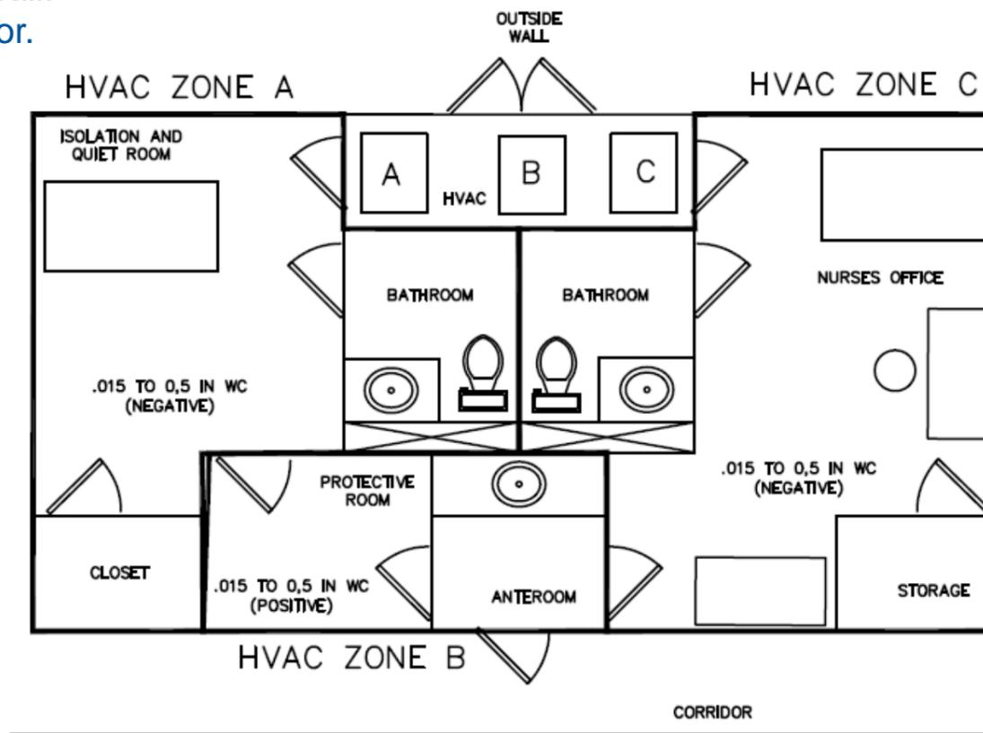
**Note:** Systems A, B, and C are the Dedicated "Isolation Mode" systems, each system is individually operated and controlled. The Supplementary HVAC systems for "Normal mode" are not shown.
