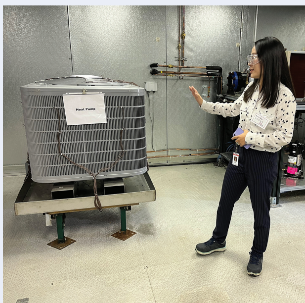
Kaimi Gao, Lead R&D Engineer/Scientist, Honeywell Advanced Materials, discusses the test setup of a residential heat pump system in the outdoor test chamber.
