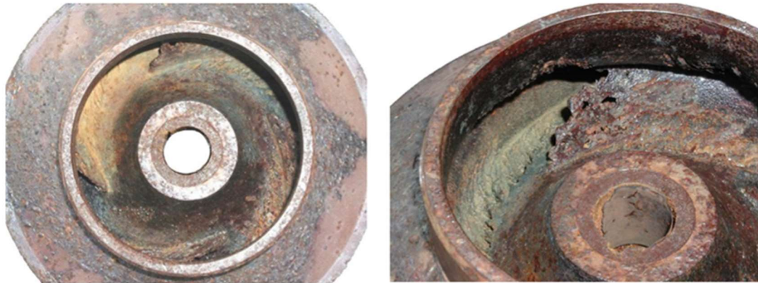
Online Figure 1 – Impeller Damaged by Cavitation (image courtesy Kelly Cramm).
