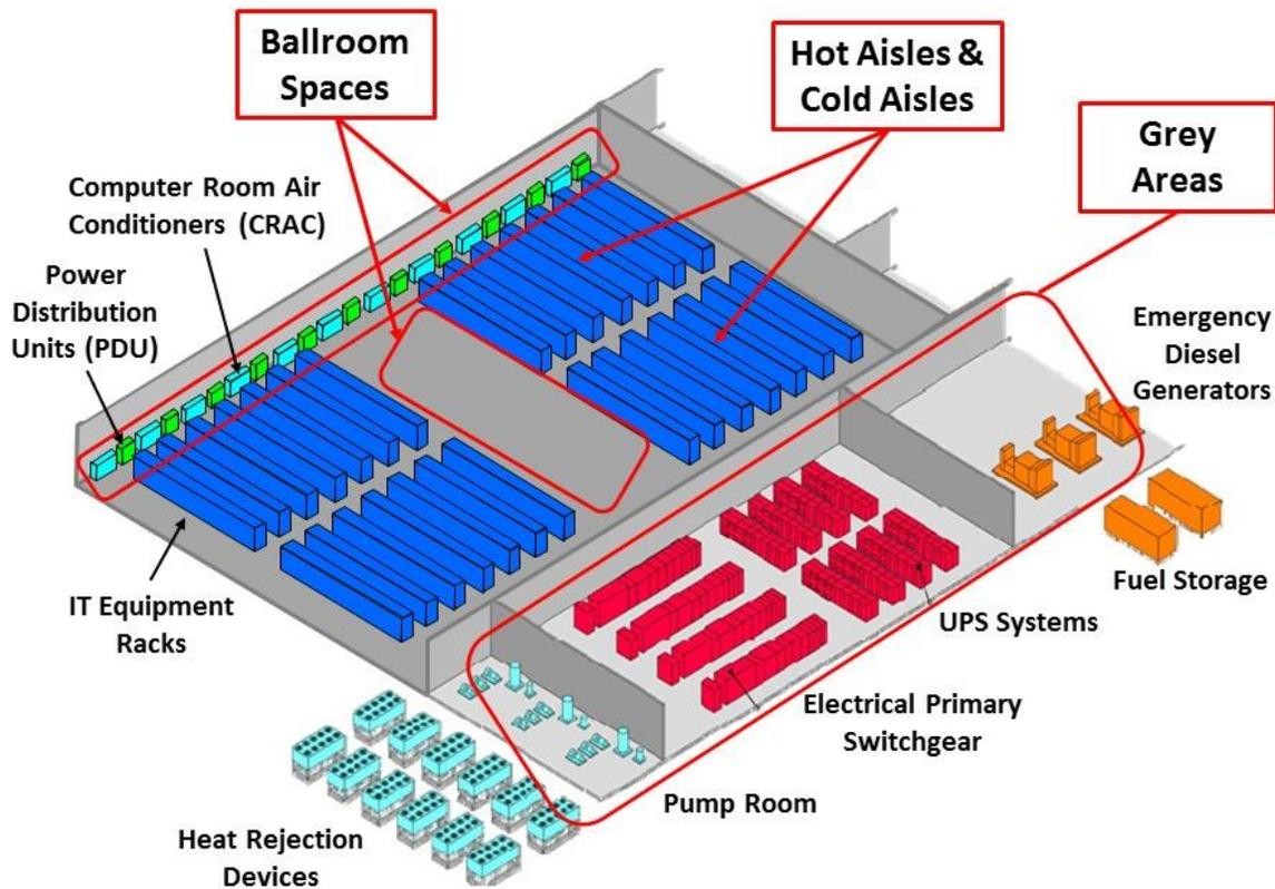
**Figure 2** General classification of data center spaces: ballroom, hot aisles, cold aisles, and grey areas.
