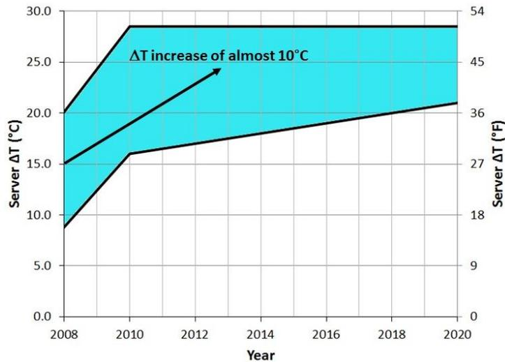
**Figure 6** Server ΔT projection at 25°C (77°F) server inlet temperature [15].
