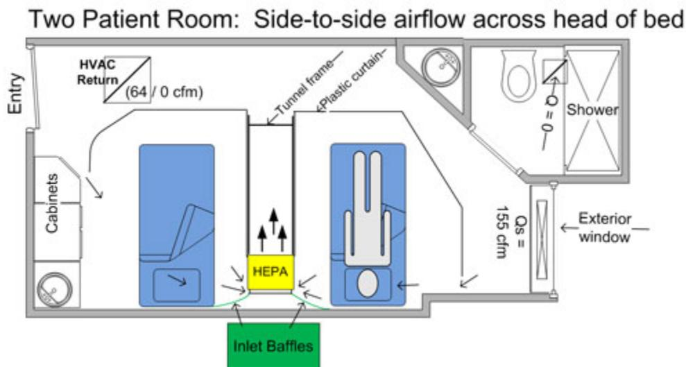
**Figure 2.** Example schematic of a two-patient expedient patient isolation room configuration. In this configuration, the occupied inner isolation zone shows the make-up air gap and HEPA filter exhaust inlet positioned to induce directed airflow across the head of patient's bed. A pvc-framed tunnel was erected near the HEPA outlet to facilitate HEPA exhaust discharge without disrupting plastic curtains.
