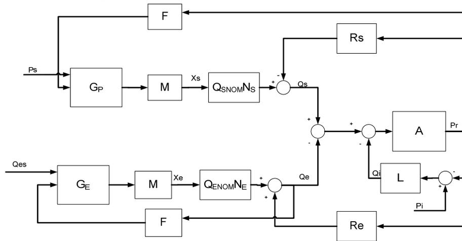
Figure 6: Block diagram of the linearized mathematical model of the room pressure feedback system
