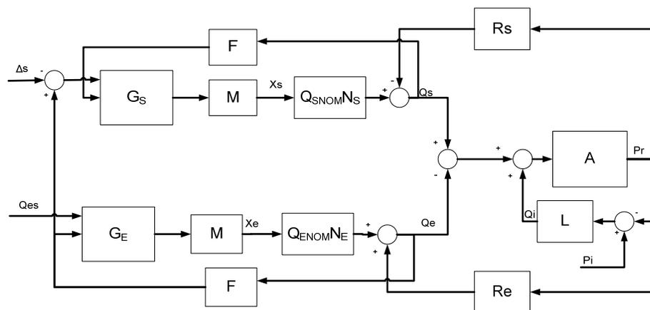
Figure 5: Block diagram of the linearized mathematical model of the flow offset control system
