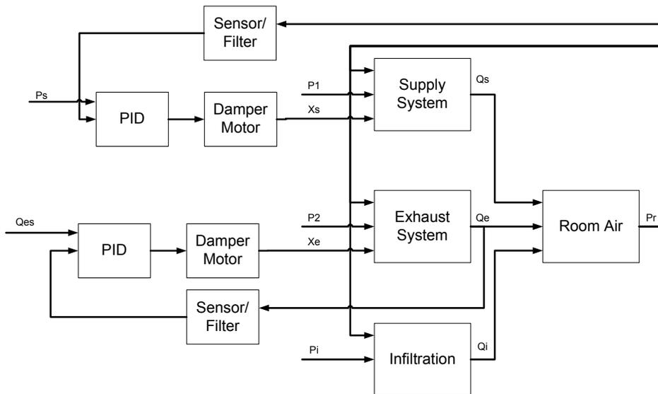
Figure 3: Block diagram of the complete mathematical model of the pressure feedback control system
