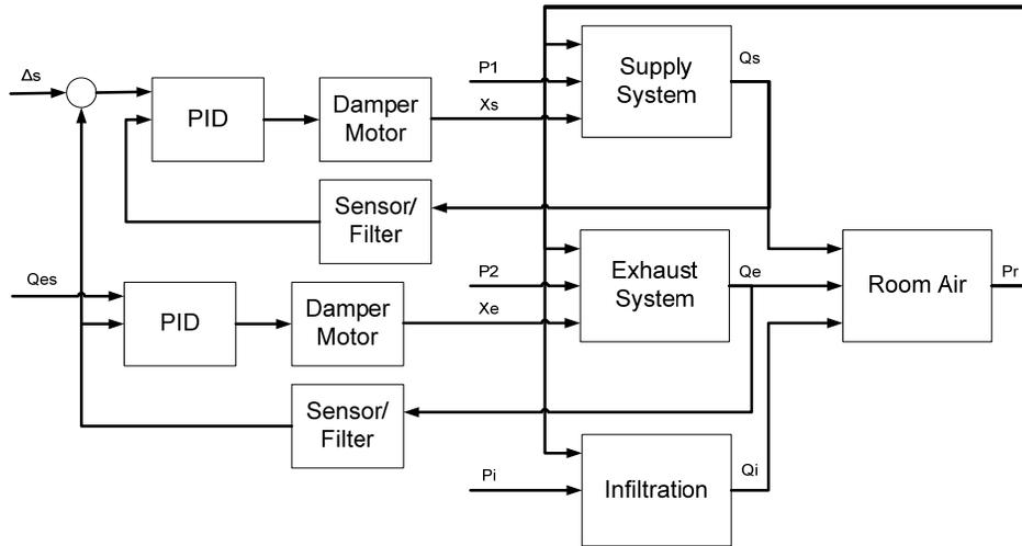
Figure 2: Block diagram of the complete mathematical model of the flow offset control system
