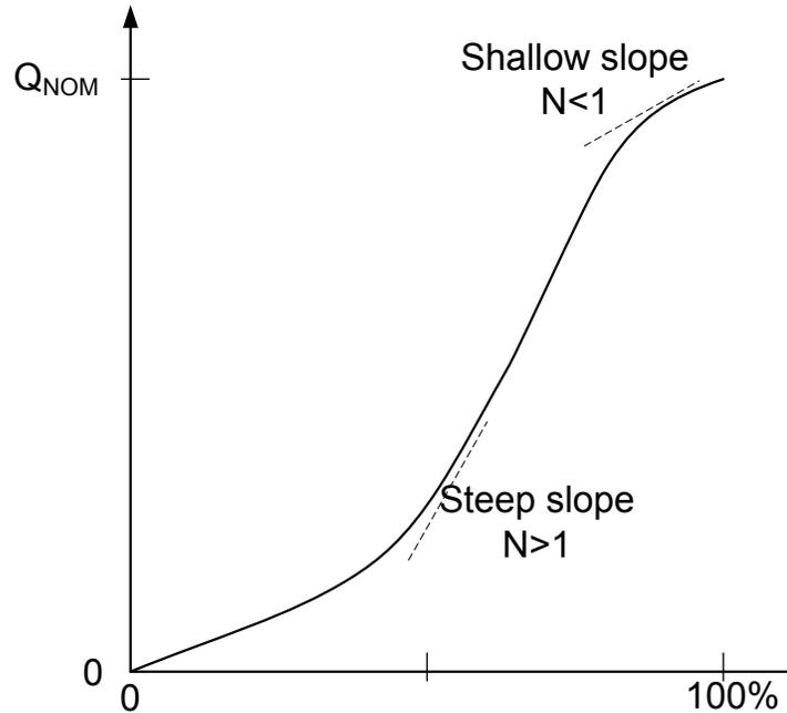
Figure 4: Non-linear damper curve and approach to linearization for analysis
