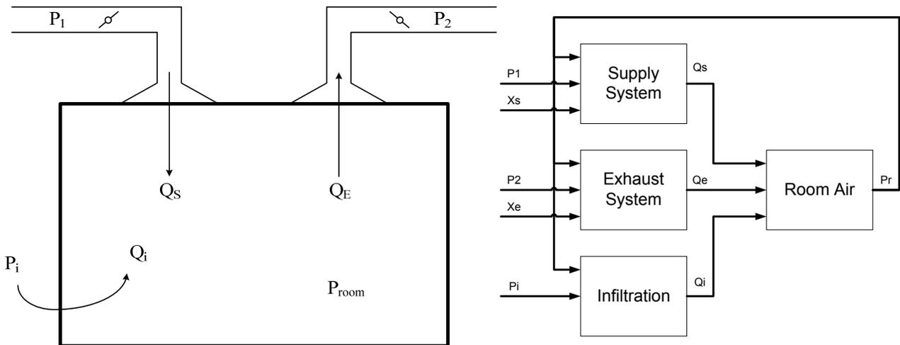
Figure 1: Schematic diagram identifying air flows and pressures in the mechanical model and block diagram illustrating structure of the corresponding mathematical model.
