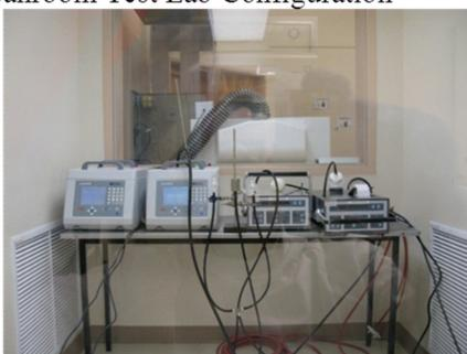
c. Particle concentration testing in Cleanroom
