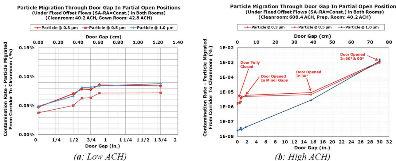
**Figure 11** CR value when cleanroom door is partially opened with a small air gap.
