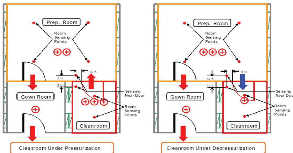
**Figure 2** Protocol of particle sensors' locations in the study (suite of three cleanrooms).
