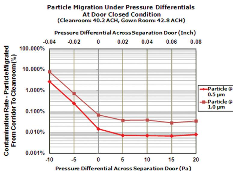
Figure 8 CR values across a closed door under pressure differentials.
