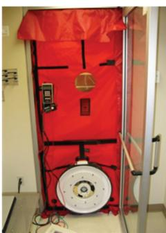
g. Cleanroom “background leakage” test with blower door to identify initial room leakage before pressurization tests by HVAC system.
