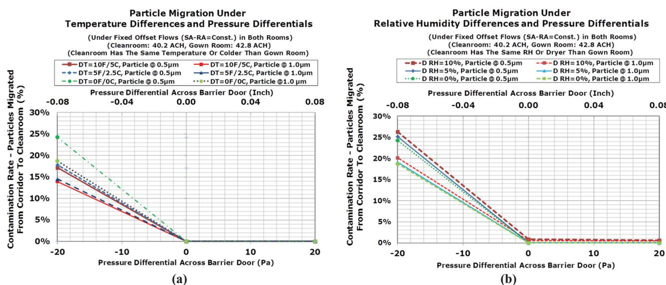
**Figure 12** Impact on particle migration (a) under temperature differential across cleanroom wall and (b) under relative humidity differential across cleanroom wall.
