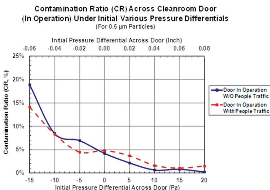
**Figure 5** The CR value during door-in-operation conditions under initial pressure differentials, with and without people traffic (Sun 2012).
