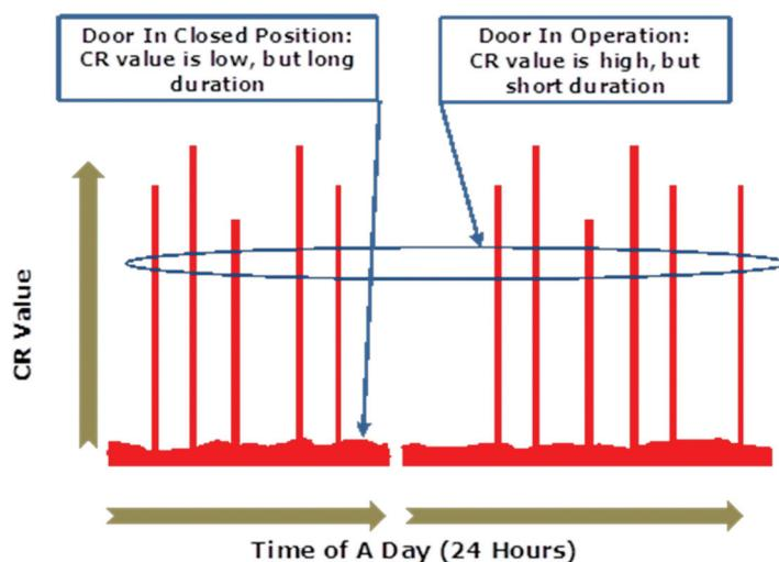
**Figure 6** Daily accumulated contamination during door-closed and door-in-operation conditions.
