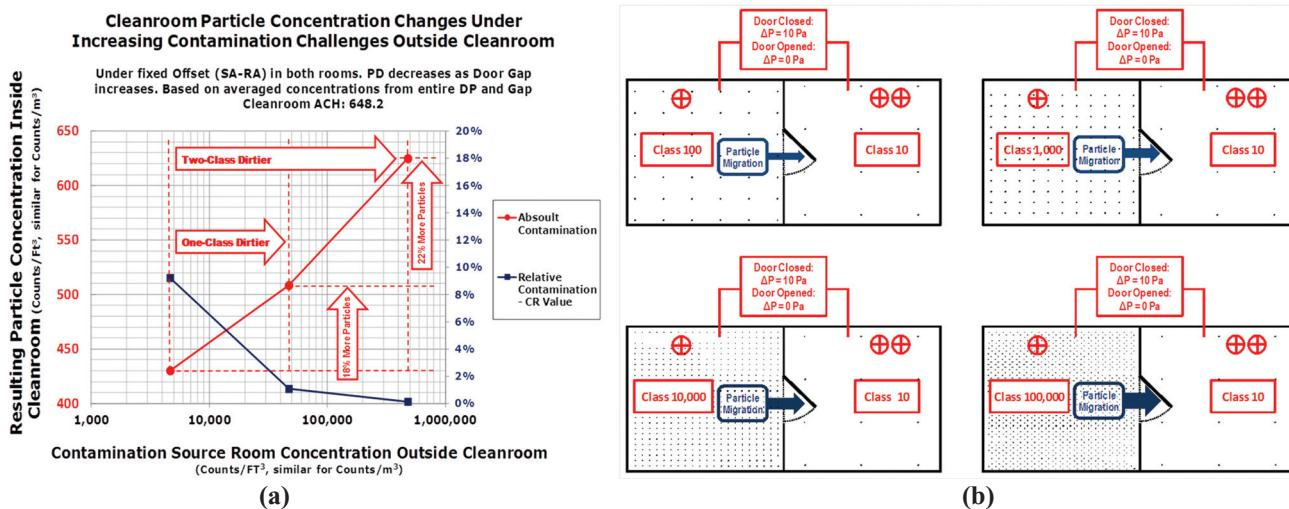
**Figure 10** (a) Cleanroom particle concentration change when contamination level increases in adjacent area across door and (b) transport of more particles (mass diffusion) into cleanroom when adjacent area is much dirtier.
