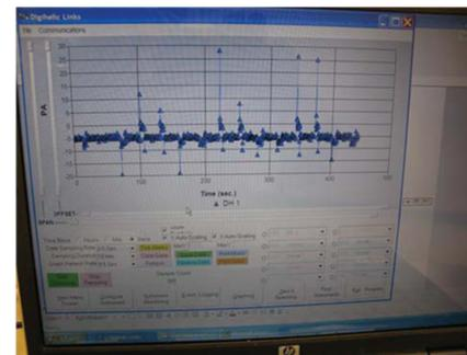
f. Fast sampling data acquisition system to analyze pressure fluctuations
