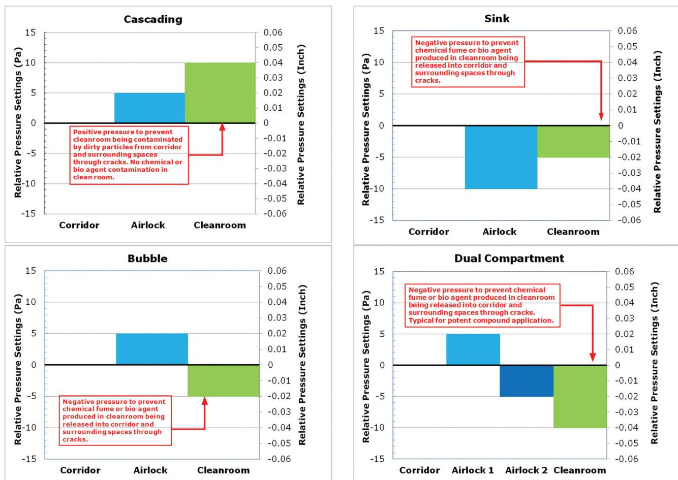
**Figure 9** Minimum pressure differential values for airlock rooms (Sun 2012).
