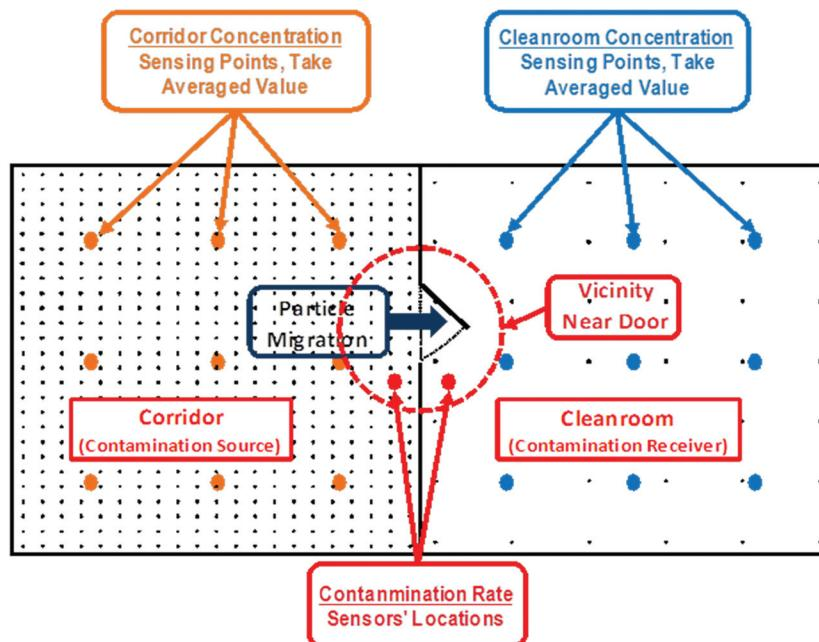
Figure 3 Contamination ratio versus concentration ratio.
