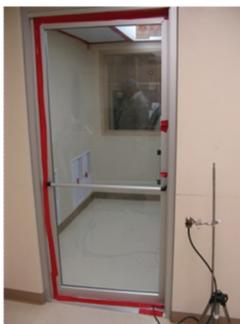
e. Room background leakage testing by airflow control devices when ceiling and door are sealed
