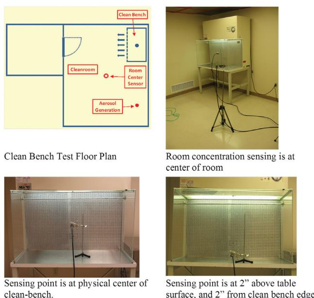
**Figure 2** Photos during clean bench tests.
