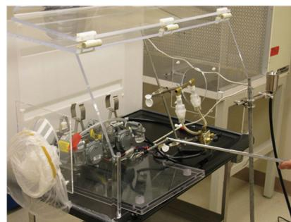
Particle generation maintained at the same level above the pressure stabilizer and outside the door.
