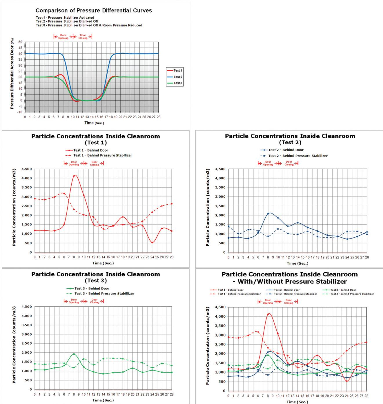
**Figure 7** Pressure stabilizer test results.
