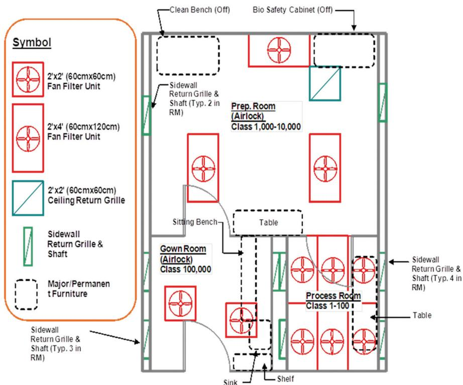
**Figure 1** Cleanroom test lab configuration.
