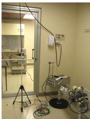
Gown Room is used for particle generation to challenge cleanroom when door is opened.
