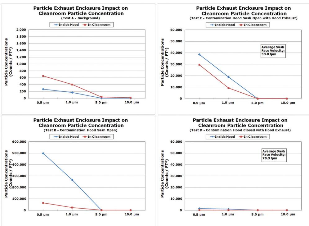
**Figure 5** Containment enclosure test results.
