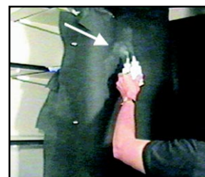
Figure 4 (left): Door opening out of positive room, smoke is contained. Figure 5 (right): Smoke plume is not captured at a negative room \Delta P of 0.001 in. w.c. (0.249 Pa). Arrow points to leading edge of plume.
