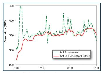
**Figure 4:** A fossil power plant following a regulation command signal.<sup>5</sup>
