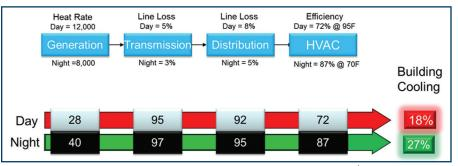
Figure 2: Relative generation source fuel efficiency, day and night.<sup>4</sup>
