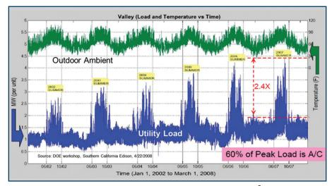
Figure 1: Typical utility load as a function of outdoor temperature.<sup>2</sup>
