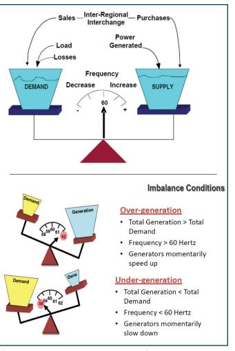
**Figure 3a (top):** Supply and demand factors impacting grid balance. **Figure 3b (bottom):** The impact of grid imbalance on frequency.<sup>5</sup>
