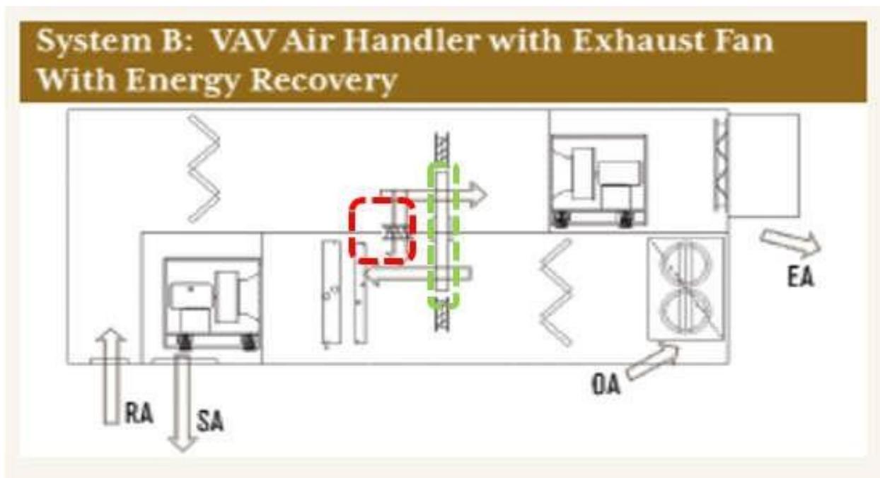
Figure 11 VAV AHU with Recirculation and ERV
