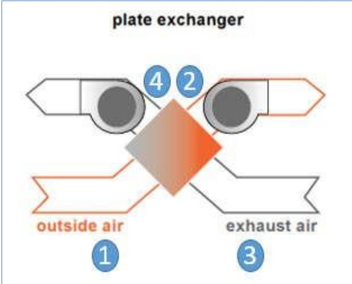
Figure 10 Airflow Layout Cross-flow Plate Exchangers
