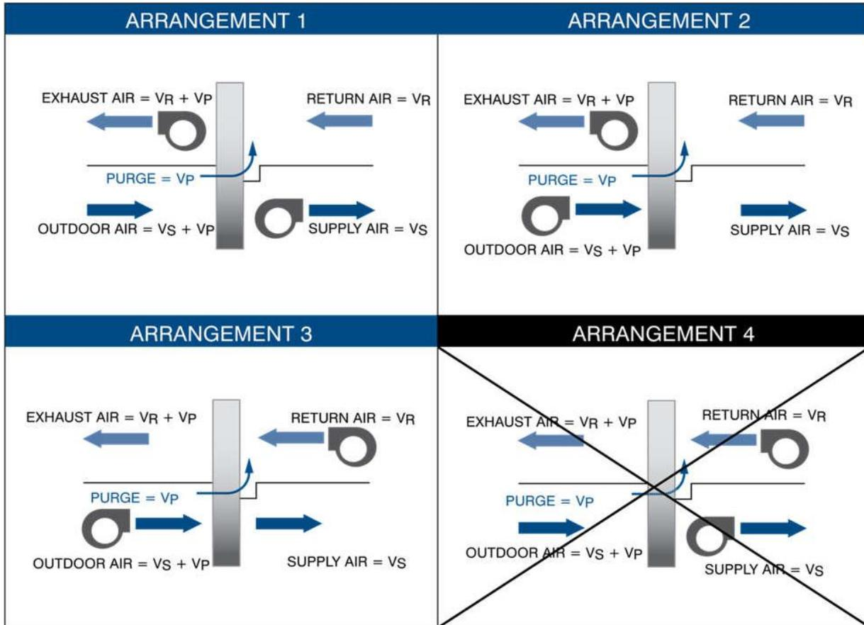
Figure 3 Fan arrangements for energy recovery exchangers
