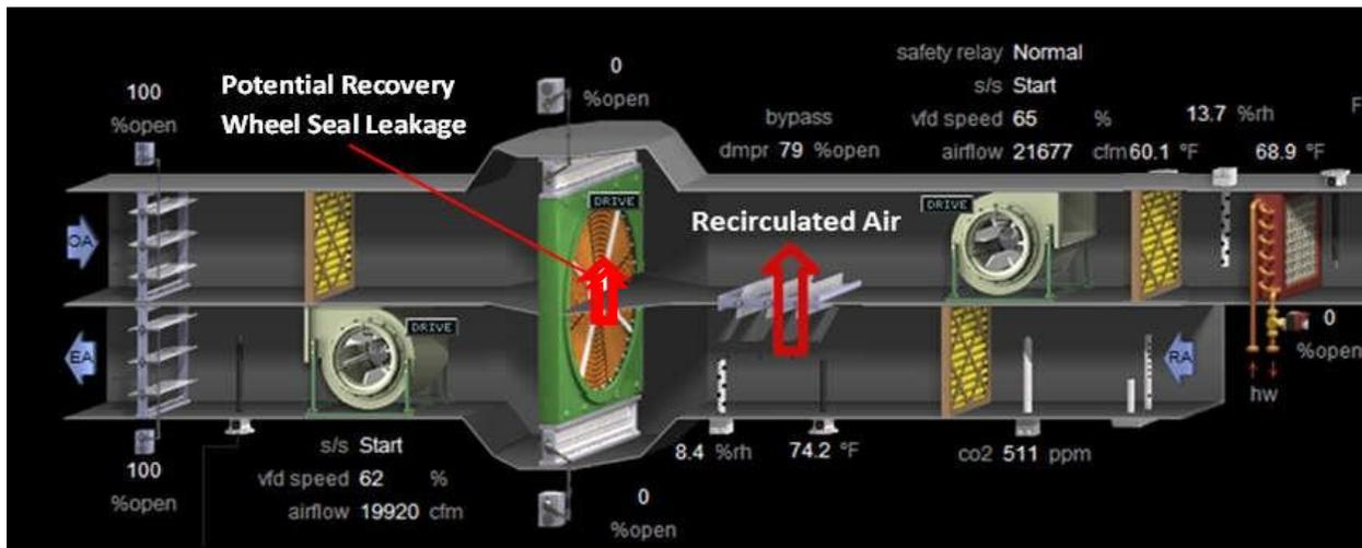
Figure 1 AHU Configuration with Recirculated Air and Energy Recovery Exchanger
