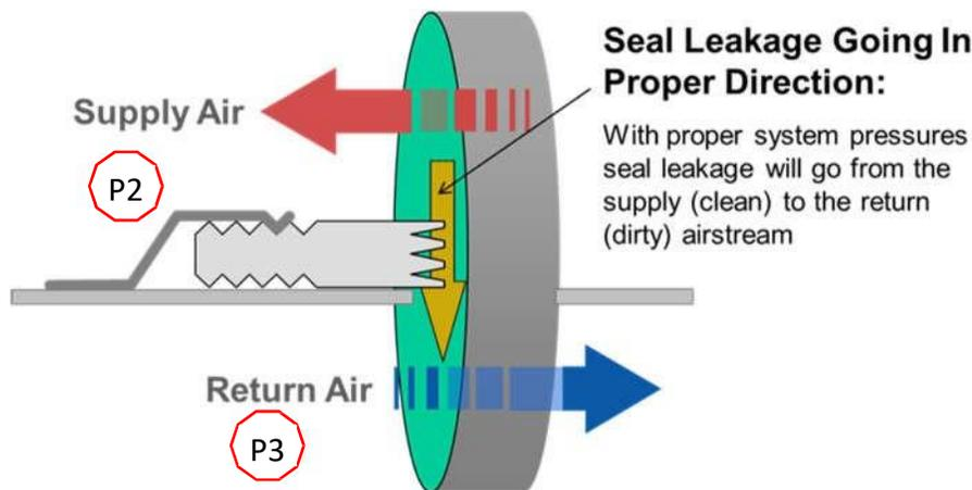
Figure 6 Supply static pressure should be higher than return static pressure.
