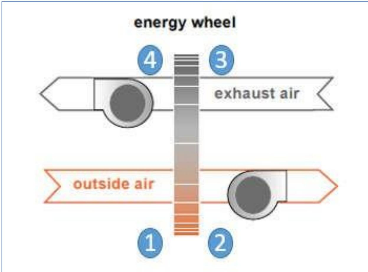
Figure 9 Airflow Layouts in Wheel Exchangers
