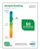
Building EQ In Operation process compares metered energy use to a baseline median EUI using the following formula: (EUI<sub>metered</sub>/EUI<sub>baseline</sub>) X 100.
