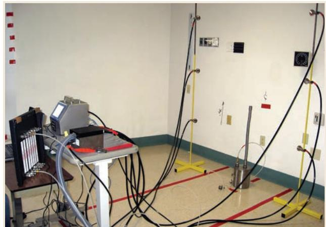
PHOTO 2 Aerosol generator & particle sampling equipment in isolation patient room.
