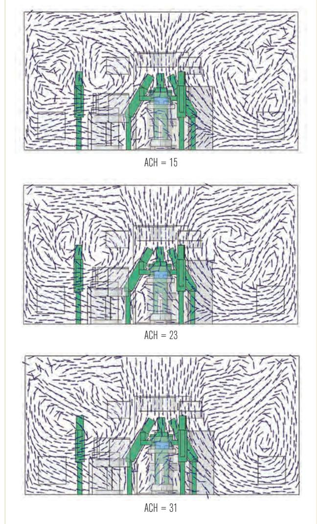
**FIGURE 3** Contours of air velocity at central plane in the operating room for three different ACH rates showing the discharge air accelerates as it approaches the operating table, with higher velocity zones (shown in red) occurring near the edge of the sterile zone at higher ACH.
