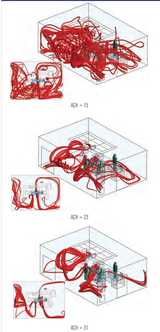
FIGURE 6 Flow path of airborne particulates originating from the anesthesiologist at the edge of the sterile zone demonstrating particles being swept from the sterile zone into the non-sterile zone before exiting the OR, at three different ACH.
