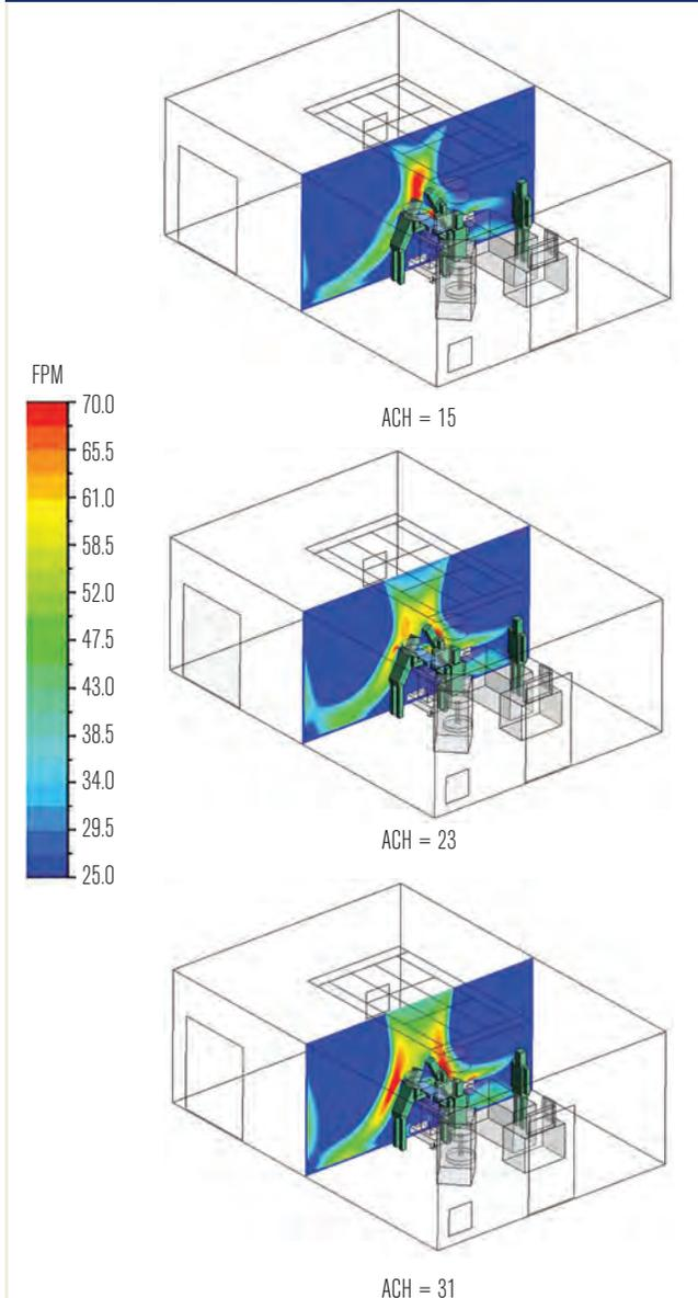
**FIGURE 4** Contours of air temperature at central plane in the operating room showing thermal stratification occurs at all three different ACH, and increasing ACH minimizes the contraction of the supply air jet and decreases the average temperature in the OR.
