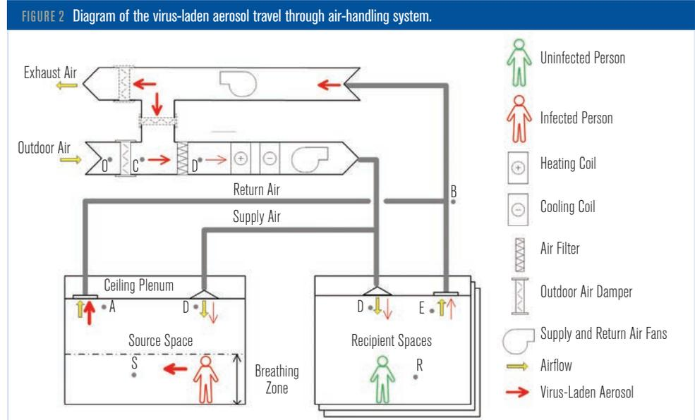
( $C_S$ ) are different and relate as follows:  $E_z = (C_A - C_D) / (C_S - C_D)$ .<sup>8</sup> The variable  $E_z$  is the zone air distribution efficiency. The concentration gradient in the recipient spaces is substantially lower than in the source space and was neglected:  $C_R = C_E$ .
