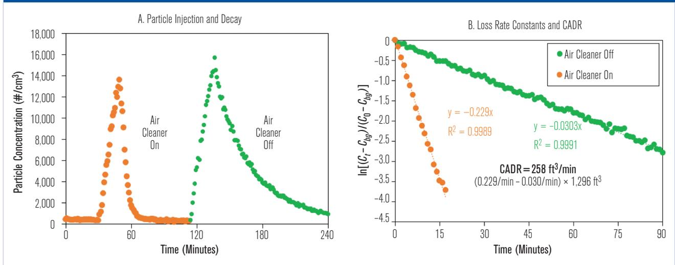
with and without an air cleaner operating. The CADR (in units of m<sup>3</sup>/h or cfm) is calculated as the difference between the two loss rate constants times the volume of the chamber (Equation 3). The CADR can also be calculated by multiplying the flow rate through an air cleaner by its efficiency, but it is not necessary to measure flow rates in Equation 3.
