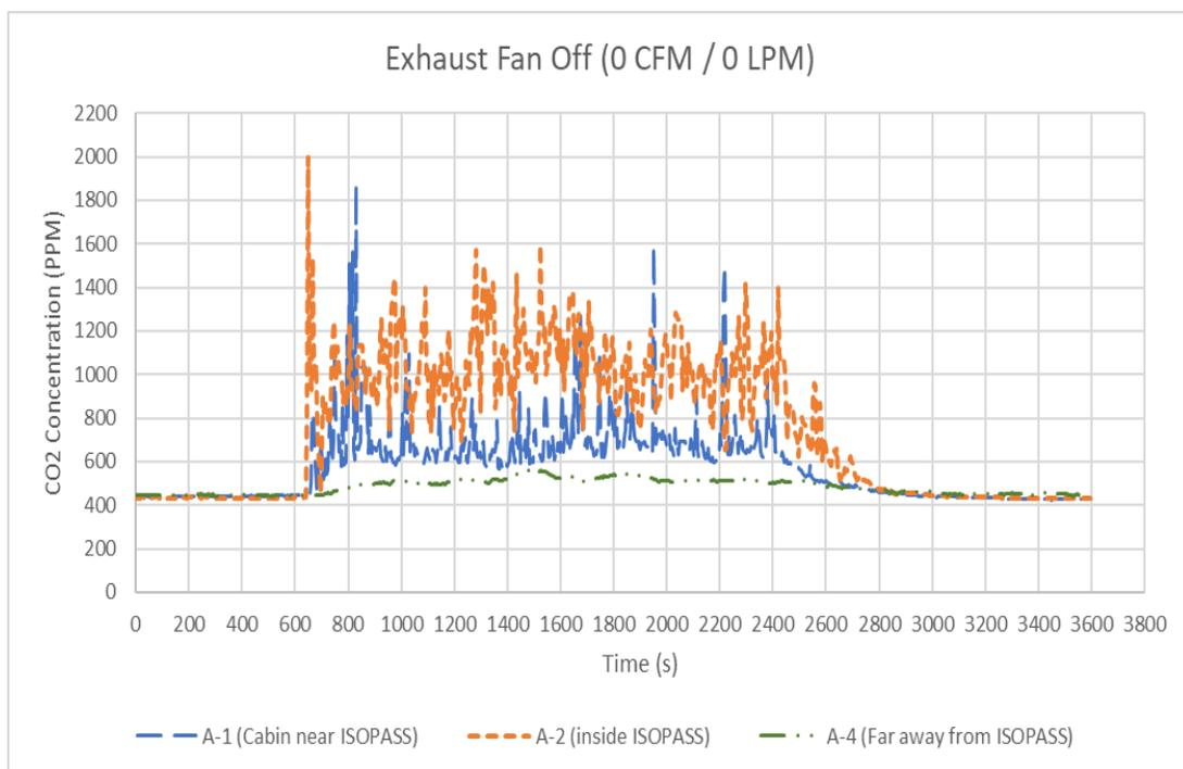
**Figure 1** Representative results with the ISOPASS off, gaspers off
