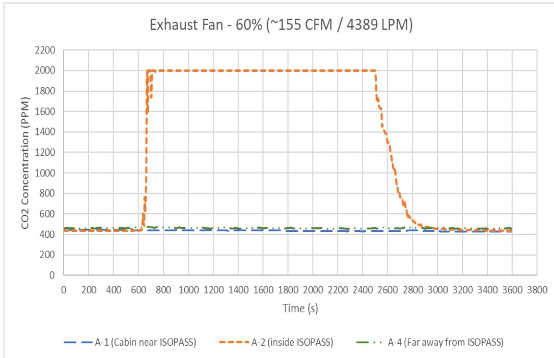
**Figure 3** Representative results with the ISOPASS on, gaspers off
