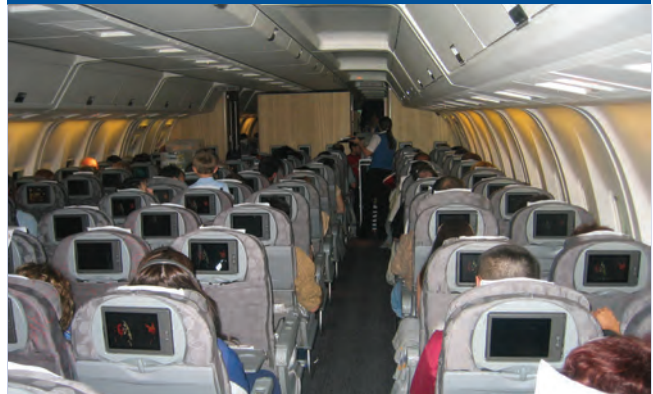
FIGURE 1 Aircraft cabins are high occupancy density, with air currents moving aerosols along four or more rows longitudinally either way, making social distancing impractical and infectious aerosol exposures more likely, while the low cabin humidity weakens our immune system's defense against infections. Humidity is kept low by ventilating with very dry outdoor air that needs to be humidified and also by the continual loss of cabin humidity from the recirculation air due to the movement of a portion of the cabin air to behind the insulation where the moisture in it condenses and freezes on the cold skin and fuselage.
