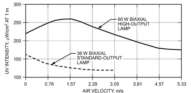
Fig. 5 Windchill Effect on Typical Low-Pressure UV-C Lamp Efficiency in Moving Airstream at 21°C
