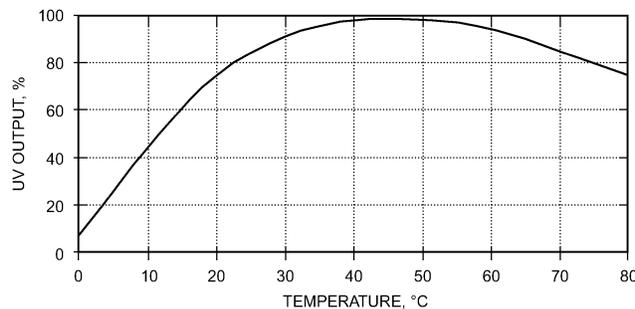
Fig. 4 Example of Lamp Output as Function of Cold-Spot Temperature
