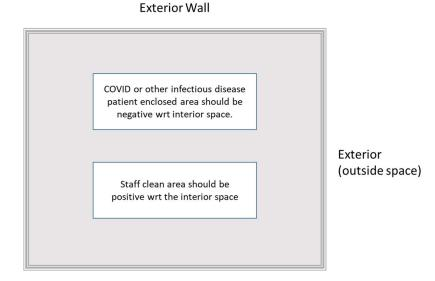
Figure 2-9: Interior zone without a perimeter zone
