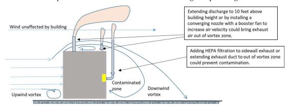
Figure 2-10: Air discharge without exhaust air filtration
