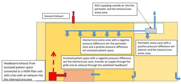
Figure 2-5: Schematic A of Enclosed Patient Room Ventilation
