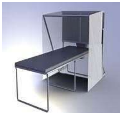
Figure 3-11: NIOSH Ventilated Headboard.
