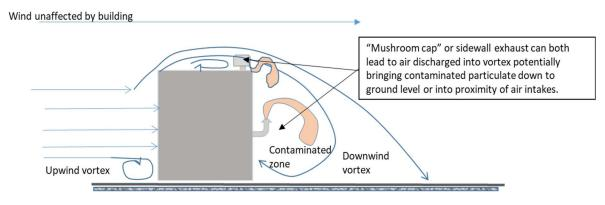
Figure 2-11: Air discharge with air filtration
