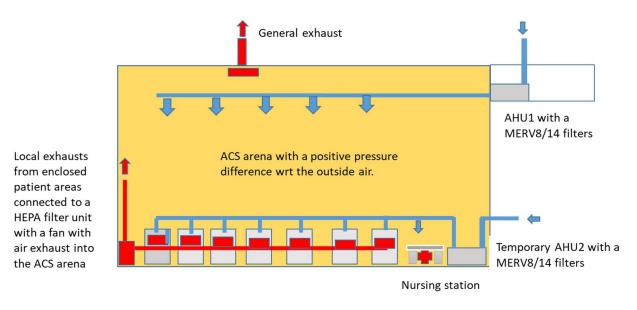
Figure 3-2: Diagram of scenario for existing and temporary AHUs for enclosed patient spaces
