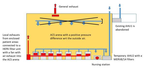
Figure 3-3: Diagram of scenario for temporary AHU servingb enclosed patient spaces
