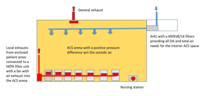
Figure 3-1: Diagram of scenario for existing AHU serving patient spaces
