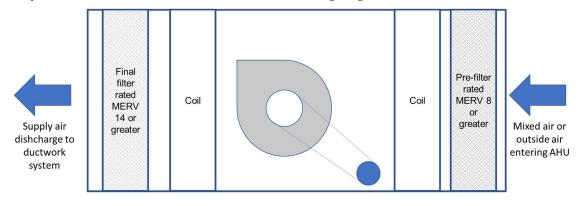
Figure 3-14: Basic diagram of AHU filter banks
