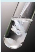
(a) Precipitation of group 1 cations by adding HCl(aq): \text{AgCl(s)} + \text{Hg}_2\text{Cl}_2\text{(s)} + \text{PbCl}_2\text{(s)}
