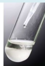
(d) Confirmation test for lead by adding HCl(aq): \text{AgCl(s)}
