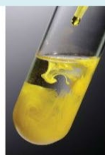
(b) Confirmation test for silver by addition of \text{Na}_2\text{CrO}_4\text{(aq)} : \text{PbCrO}_4\text{(s)}
