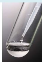
(c) Confirmation test for mercury by adding \text{NH}_3\text{(aq)} : \text{Hg}_2^{2+} + \text{Hg(NH}_2\text{)Cl(s)}
