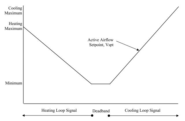
Figure 5.5.5 Control logic for cooling-only VAV zone.
