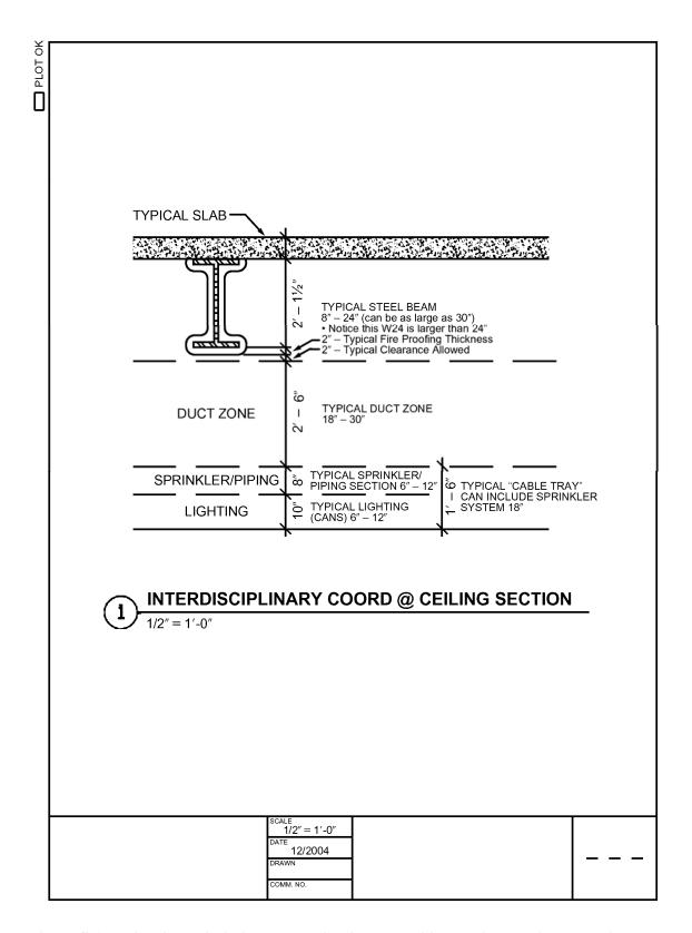
Figure S-1 Typical interdisciplinary coordination and ceiling section detail on drawings.
