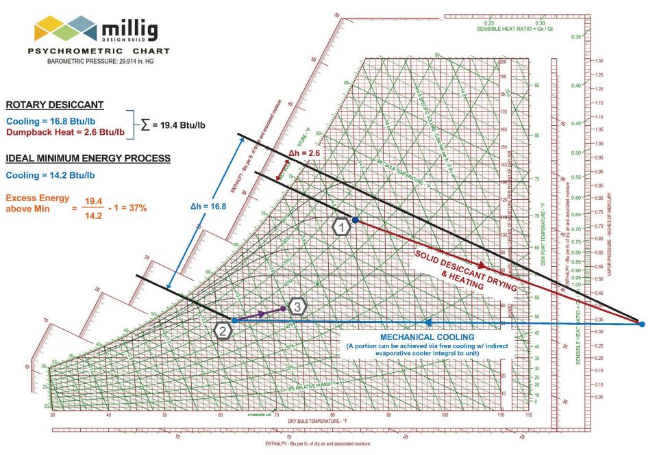
Compare this to an application where higher temperature, low humidity supply air is desired. In Psychrometric Chart 5, the desired supply air conditions are ( $\langle 4 \rangle$ ), 85°F temperature, 49°F dew point. Again, it is important to establish the theoretical minimum cooling energy required to achieve the given conditions.
