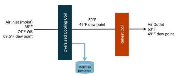
**Dehumidification Control via Overcooling and Reheat**
