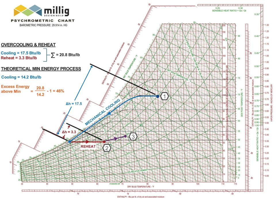
In Psychrometric Chart 2, 49°F dew point air is needed to absorb the moisture needed to maintain 50% RH in the space. However, this 50°F air, if delivered to the space without reheat, would result in an overcooled space and too high of relative humidity. Consequently, reheat is needed to add 13°F of sensible heat to result in the needed space conditions of 72°F and 50% RH.
